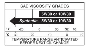
**NOTE:** Although multi-viscosity oils (5W30, 10W30 etc.) improve starting in cold weather, these multi-viscosity oils will result in increased oil consumption when used above 32°F. Check your engine oil level more frequently to avoid possible engine damage from running low on oil.
